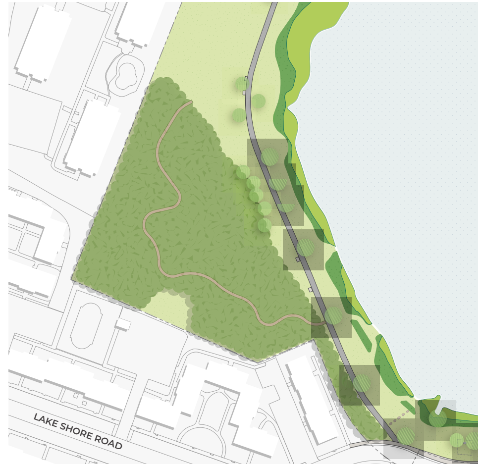
FIGURE 4.12 CONCEPTUAL PLAN FOR THE WOODLAND ACCESS TRAIL A woodland path would create a unique experience of the park and provide informal monitoring of the area, deterring illegal dumping and the unchecked spread of invasive species.
