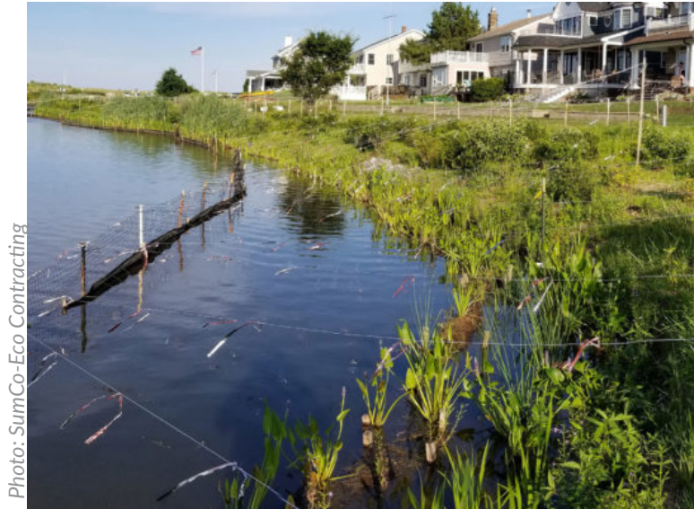
FIGURE 4.7 EXAMPLE OF OVERHEAD HERBIVORY FENCING (LEFT) AND PLANT ESTABLISHMENT FENCE (RIGHT) Fencing provide enough time for new plantings to get established without interference by humans or grazing geese. Overhead fencing uses strings and mylar tape to deter geese from landing. In-ground fencing protects new plantings from humans and some grazing wildlife. Raising the fence several inches above ground level permits amphibians and reptiles to move through the fencing, but also reduces protection from small mammals, such as rabbits.
