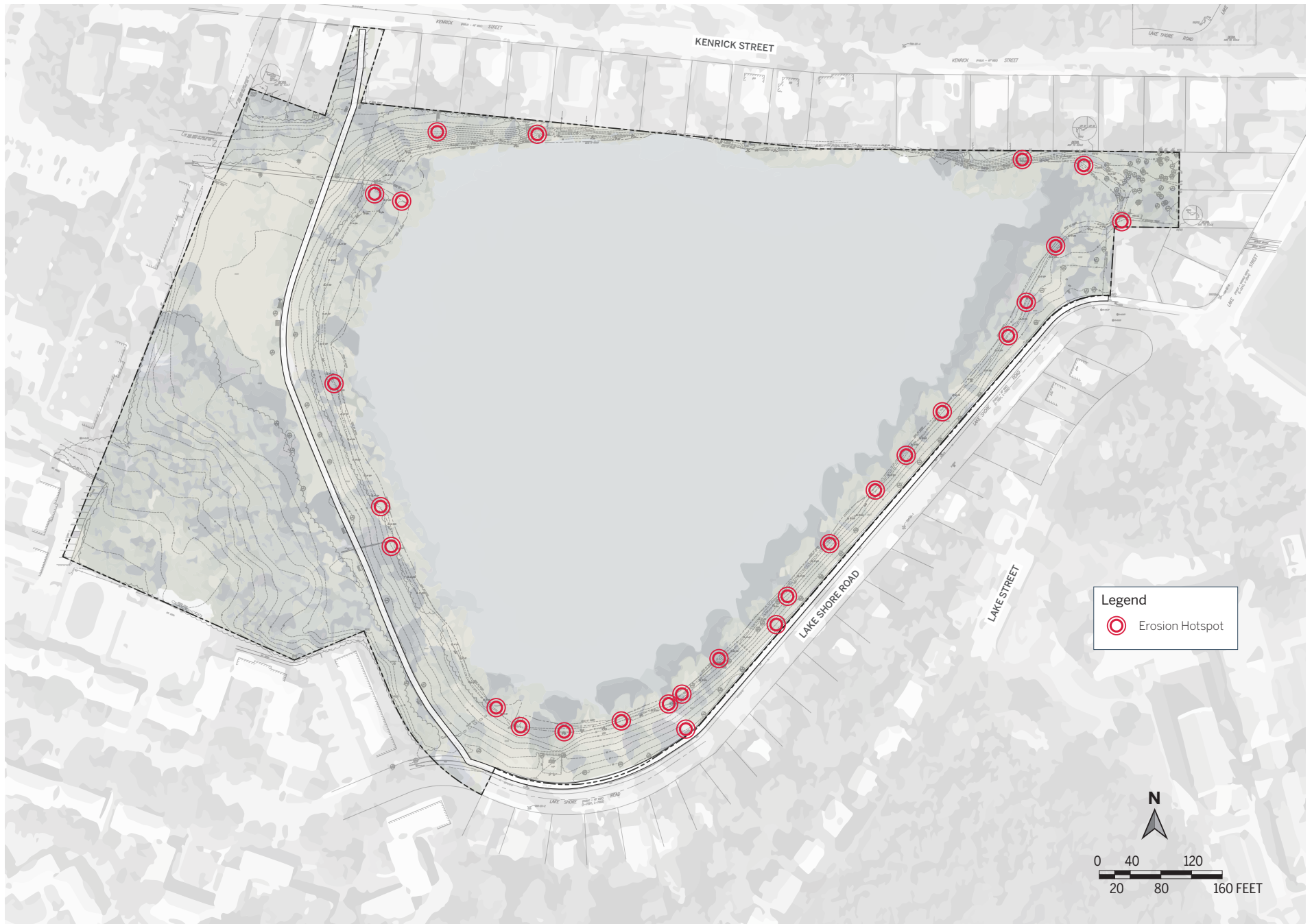
FIGURE 2.18 EROSION HOTSPOTS AT CHANDLER POND
